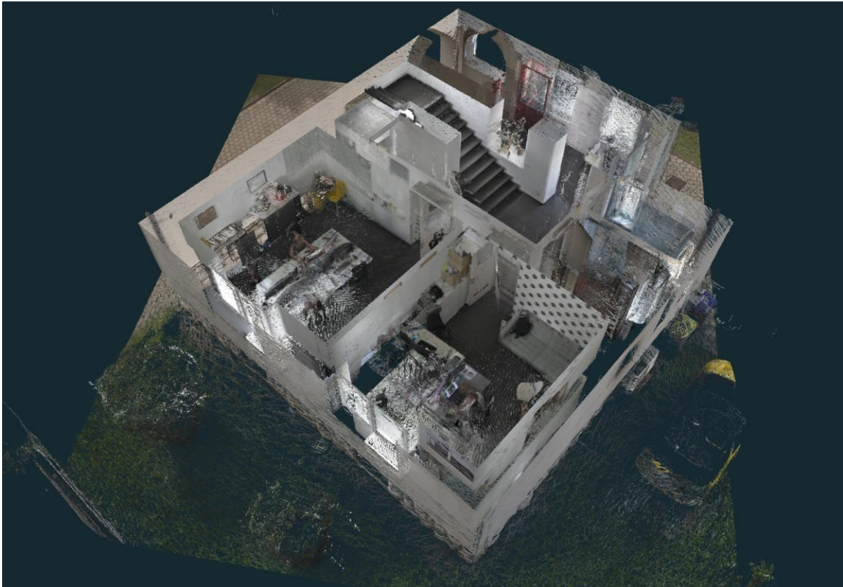
Bounding box inspection of an office building in 3Dsurvey.
