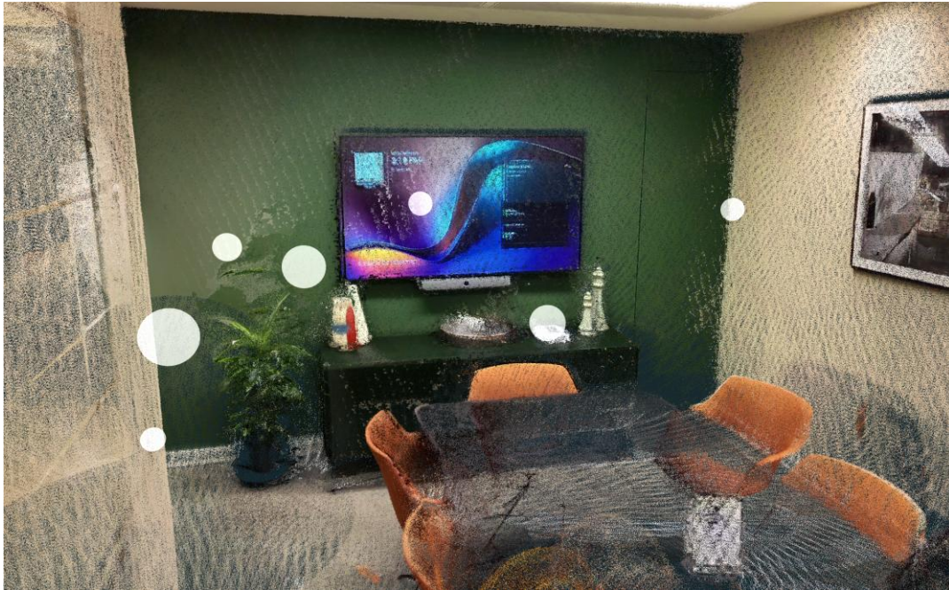
A quick office scan highlighting both the strengths and limitations of the FJD Trion P1 point cloud.
