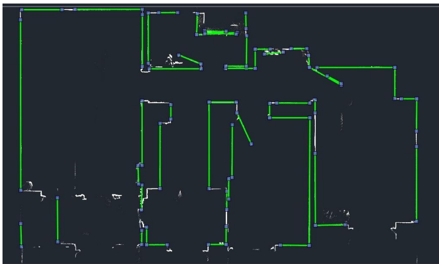
A simple floorplan of an apartment with automatic line detection.
