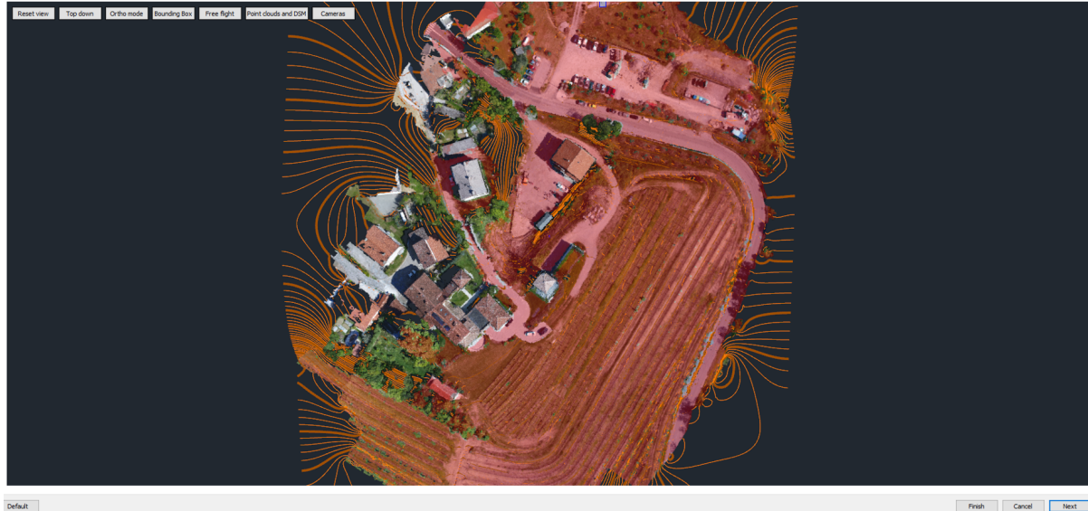
Figure 2: Points marked and filtered by increased values of Terrain Elevation and Terrain Slope
